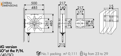
For the SWIVELLING version add the suffix "/SO" at the P/N. For example: 440/40/SO
